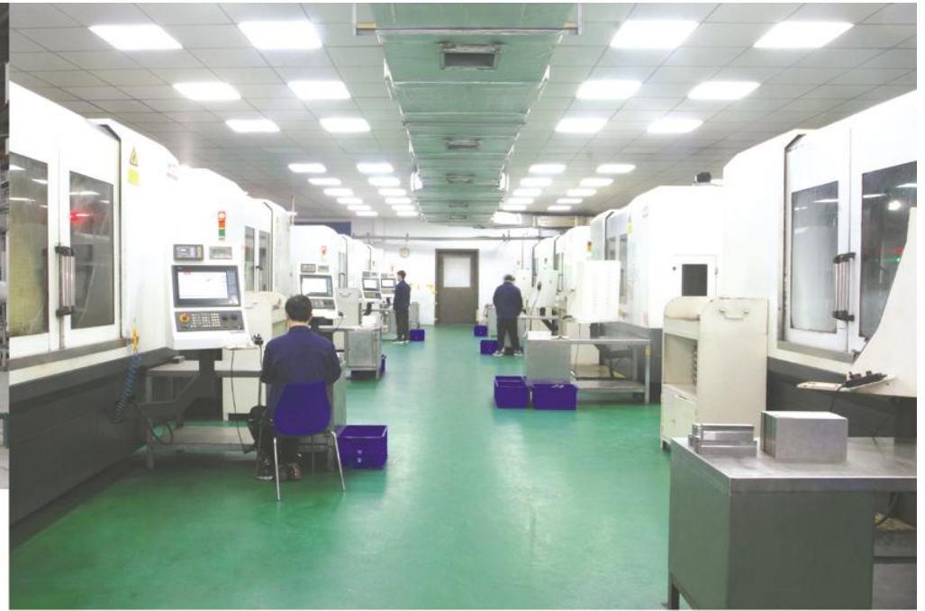
▲ GRINDING EQUIPMENT WITH UPDATED CNC COMPUTING SOFTWARE FOR AFTER HEAT-TREATMENT THREAD ROLLING DIE PLATES.
