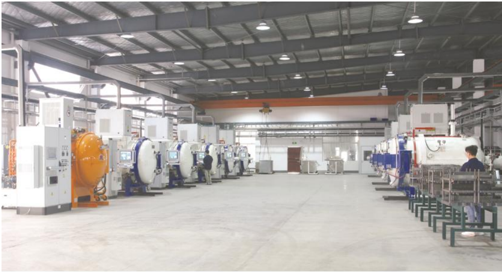
▲ HIGH-TECHNOLOGY VACUUM AND NITRIDING FURNACES ARE FROM FRANCE AND GERMANY FOR SURFACE TREATMENT
